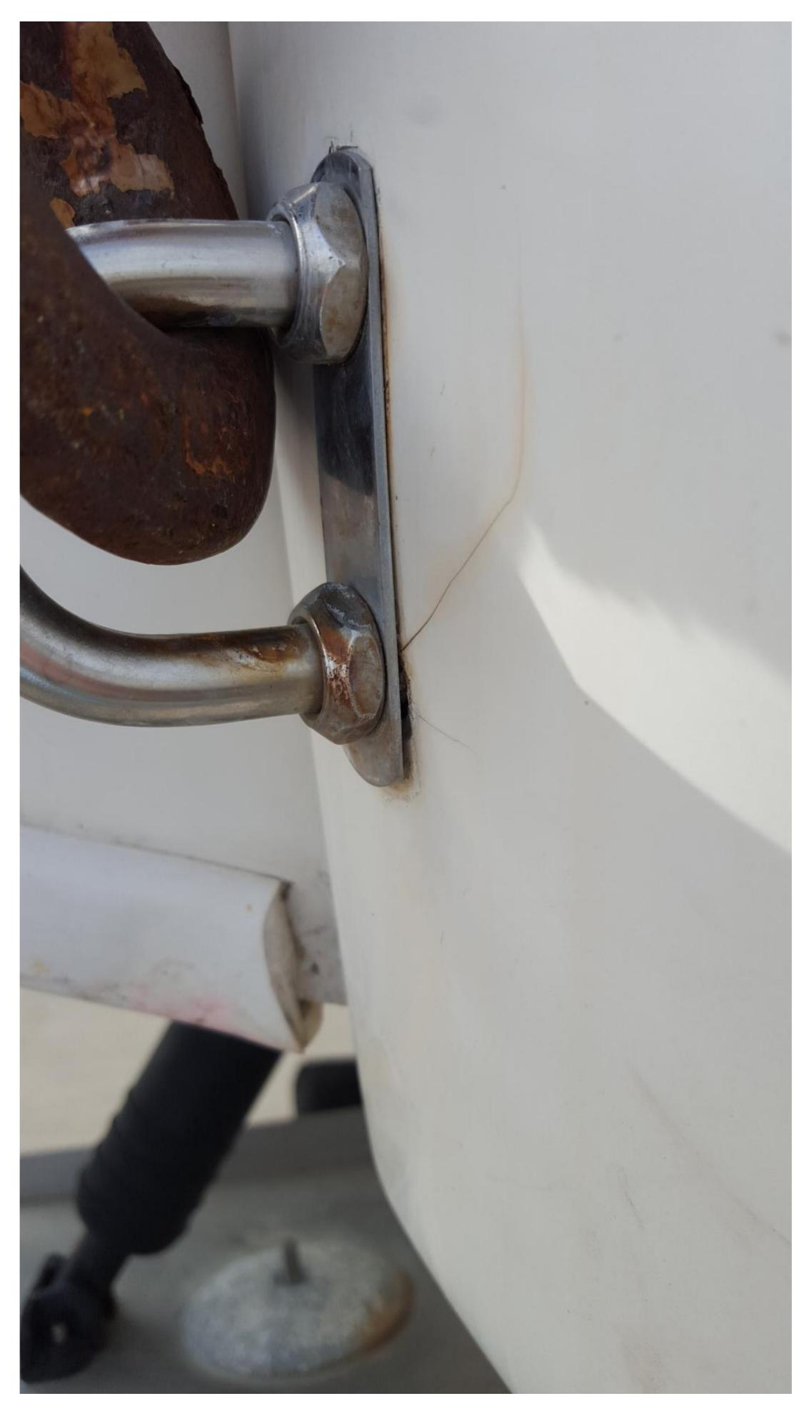
Transom Crack Fiberglass Boat
